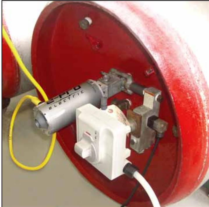
Figure 2: E-Pro® Valve Closure System installed on a ton container with a vacuum regulator.
