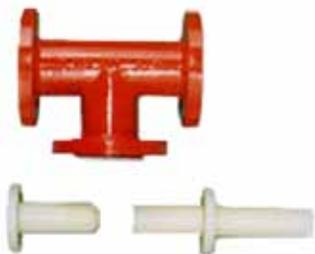
The Powell Chlorine/Sulfur Dioxide Eductor is suitable for use in liquid and gas applications and was developed to safely evacuate chlorine or sulfur dioxide cylinders, tankers, railcars, and piping systems. The unit is based on a unique manufacturing concept, and is custom sized for each application. Sodium hydroxide is typically used for the motive liquid. An optional cross design with gauge is also available. The Powell Chlorine/Sulfur Dioxide Eductor features include:
