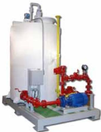
The Powell ProVent Chlorine/Sulfur Dioxide Equipment Scrubber is designed to evacuate transfer hoses, piping, and vaporizers used for chlorine process systems. The Powell ProVent, which can be sized for your specific needs, recirculates a caustic soda solution through an eductor to safely neutralize any chlorine remaining in the hoses or piping. In case of power failure, the scrubber can still neutralize chlorine sulfur dioxide under pressure. Other features of the Powell ProVent include:
